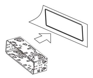
Bend as many claws outward for tight fit, to lock the sleeve into place.
