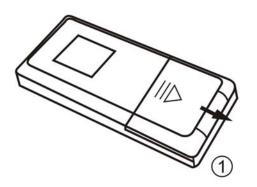
2. Place the new battery in the tray and slide the cover back into place.
