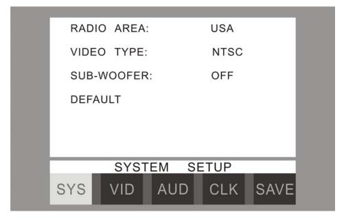
RADIO AREA: USA – JAPAN – OIRT – EUROPE – ASIA – USA VIDEO TYPE: NTSC SUB-WOOFER: OFF – 80 HZ – 120 HZ – 160 HZ DEFAULT: the unit will restore all default settings of Sound Parameter, Picture Parameter & Tuner Parameter.
