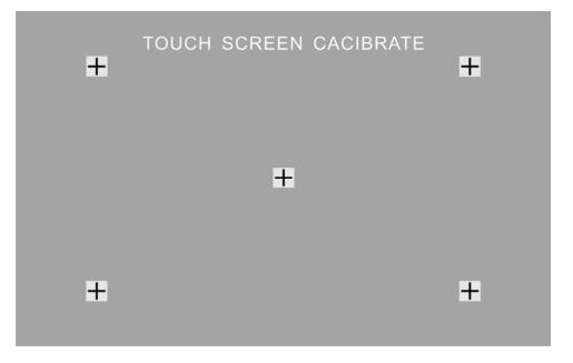
After all 5 points change to brighter, the unit would finish the CALIBRATE and power off again. Then the Touch Screen is restored to their default positions.
