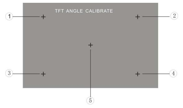
To touch the points from 1 to 5 until the points change to brighter by using a ballpoint pen or pencil.
