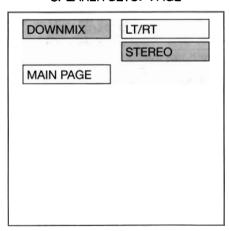
This is to activate the audio output from DOLBY AC3 5.1 DOWNMIX to 2 channel mode. Select the preferred SPEAKER connection by using the cursor buttons.
