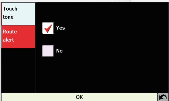
This function allows you to alter the audible alerts provided during navigation and to turn the audible beeps on/off while selecting functions on the display.
