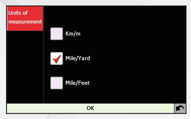
This menu allows you to display between metric and imperial measurement. Ingenix has 3 units of measurement.
