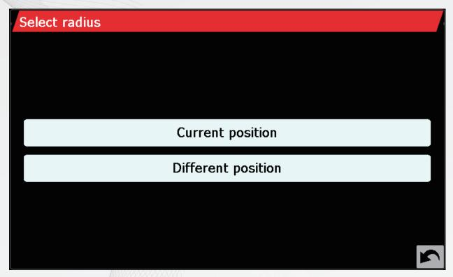
The basic function of "Find by nearest POI" is similar to "Find by POI" you can search the POI located near your current position by using "Current position". In "Find by nearest POI" however you can also search for POI's near a different location.
