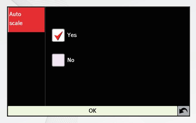
"Auto scale" function automatically magnifies the map as you approach a junction or intersection, where you may need to turn, This function can be turned on/off as you wish by pressing the check box. And press "OK" button.
