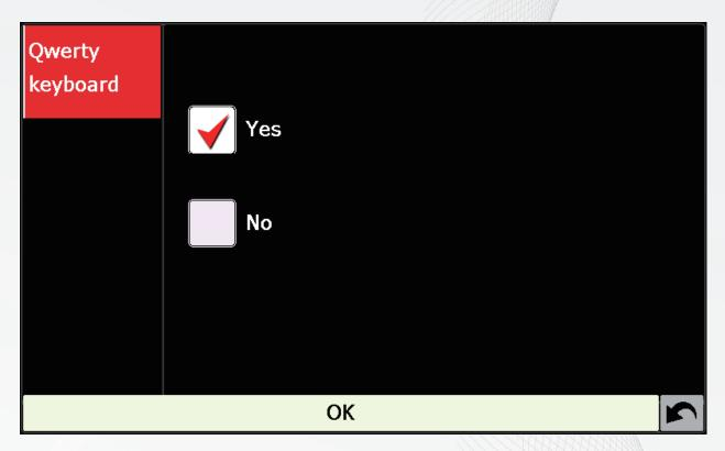
You can select whichever mode is more convenient for you in this menu. Ingenix has two kinds of keyboard. The one is an basic type keyboard listed in alphabetically and the other is Qwerty keyboard. The Qwerty keyboard is the standard keyboard you would find on a computer keyboard.
