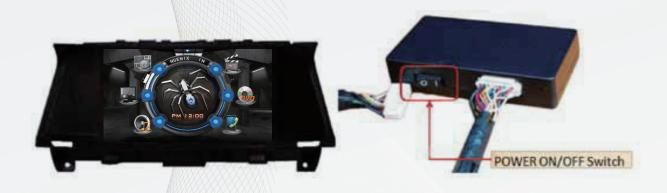
→ Honda Model has Power On/Off switch back side of Control box.
