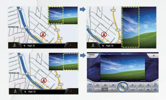
While the PIP image is in split screen. Touching the left side of the image will engage full screen view. Touching the right side of the image will engage the small screen view.
