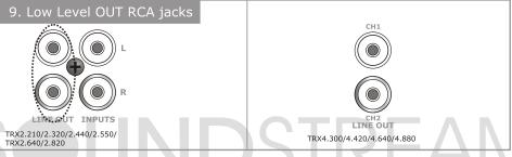
The LINE OUT allows you to build multiple amplifier systems without having to use splitter cords to distribute the signal. Now it is simply a matter of bringing one set of RCAS into the first amplifier, then using the line out RCA jacks as the feed to the next amplifier.
