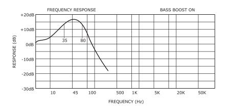
NOTE: Raising the Bass frequency allows higher frequencies to reach the bass speakers while blocking lower frequencies from midrange speakers. Lowering the Bass frequencies allows lower frequencies to reach the midrange speakers while blocking higher frequencies from bass speakers.
