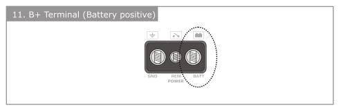
Due to the power requirements of the Amplifier, this connection should be made directly to the positive(+) terminal of battery. For safety measure, install an in-line fuse Holder (not included) as close to the battery positive(+) terminal as possible with an ampere rating; not to exceed total value of fuses in Amp.
