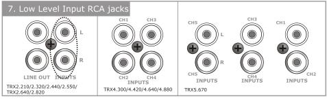
These inputs are for signal cables from the source. Always use high quality shielded RCA cables.
