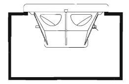
Box is given as internal air volume including driver displacement
