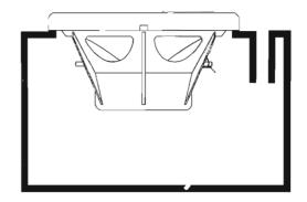
Box is given as internal air volume including driver displacement
