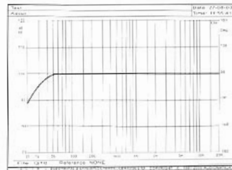
9. Subsonic filter: 50Hz; Q=1,1
