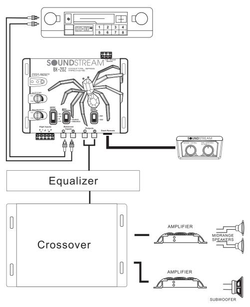
**NOTE:** For signal connection, the output RCA connectors should be connected to the next component after the BX-20Z, such as a crossover, equalizer, or amplifier. Just remember, the BX-20Z should go inline before a crossover.
